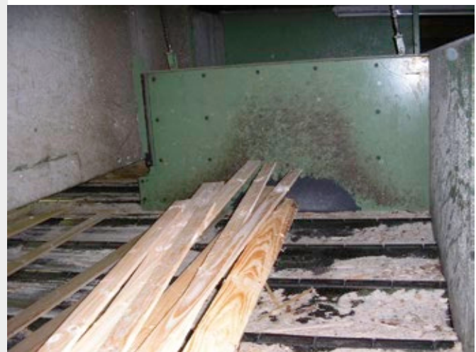
Impact protection for wooden battens
