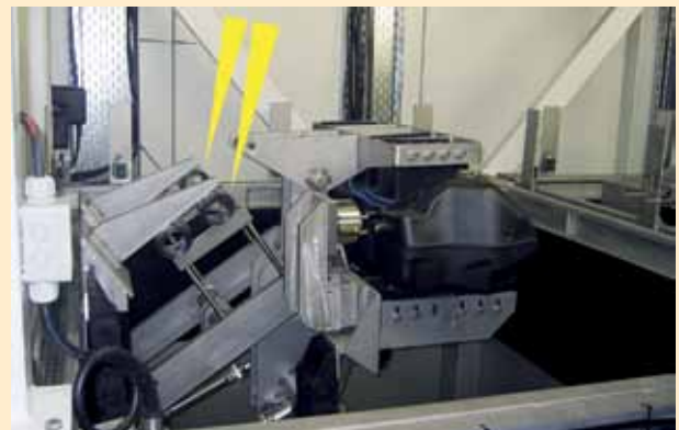
With the kind permission of Worthmann Maschinenbau GmbH Economical end position absorption on the hydraulic drive
