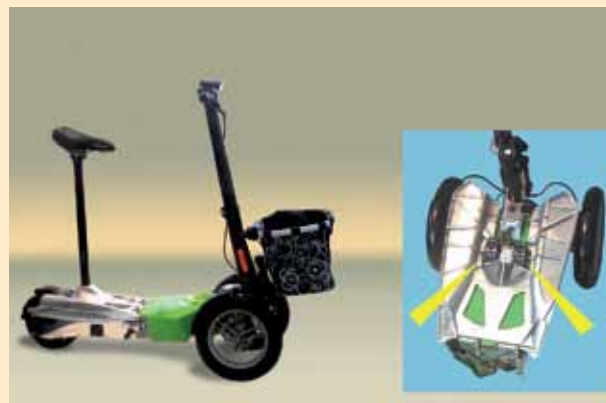
Profile dampers increase the riding comfort of an electric scooter
