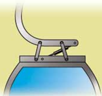
Swinging movements cushioned by hydraulic dampers
