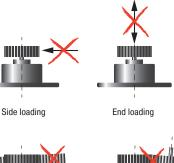
Note! The rotary axes, square mounts or free-wheel
