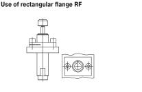
Mounting of damper in borehole with two locknuts
