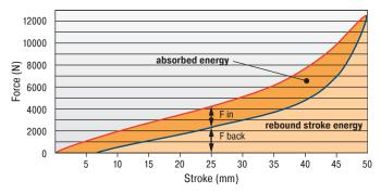
The total energy and its absorbed portion can be determined from the selection charts. Example: Energy to be absorbed 50 Nm = stroke used 25 mm see example energy stroke characteristic curve. At the force stroke characteristic curve the determined stroke can be used to determine the share of absorbed or returned force. Dynamic (v > 0.5 m/s) and static ( $v \le 0.5 m/s$ ) characteristic curves available for all types on request.
