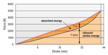
The total energy and its absorbed portion can be determined from the selection charts. Example: Energy to be absorbed 50 Nm = stroke used 31 mm see example energy stroke characteristic curve. At the force stroke characteristic curve the determined stroke can be used to determine the share of absorbed or returned force. Dynamic (v > 0.5 m/s) and static ( $v \le 0.5 m/s$ ) characteristic curves available for all types on request.
